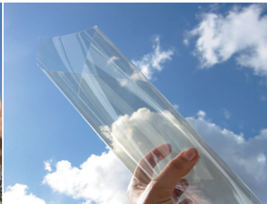
Figure 2: The transparent foil with a special coating is used to make curved surfaces sensitive. Furthermore, it can be cut in nearly any shape
